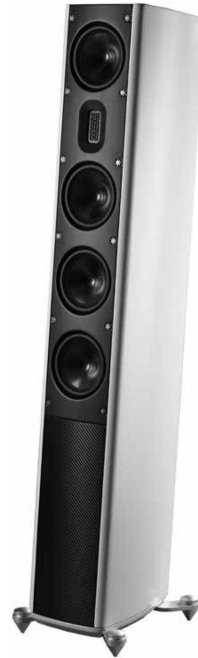
The MB5 B is a unique floor-standing speaker with four 4.5" carbon-coned drivers and a sealed ribbon-tweeter. The enclosure is heavily braced, curved and with solid carbon reinforcements. The MB5 B works as a 3-way speaker, where three 4.5" woofers handles the lower frequencies. The delicate midrange is also handled by a 4.5" carbon-coned driver and together with the ribbon-tweeter, the MB5 B is able to deliver a very crisp and transparent sound with a deep, controlled bass.
